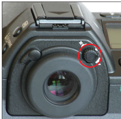
FIGURE 5.19 A diopter wheel lets you adjust your optical viewfinder to compensate for your own vision.
